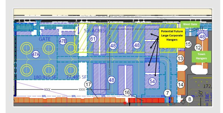
Over the years the Airport has received interest in developing corporate hangars to house large jets, therefore staff has recently taken the very first step in being able to develop additional hangars, by adding a layout to the Airport Layout Plan (ALP). Nothing can be constructed unless it is included on the ALP and approved by the FAA, so we have shown up to four large corporate hangars. No plans for development are currently underway, but we will be looking into next steps soon.
