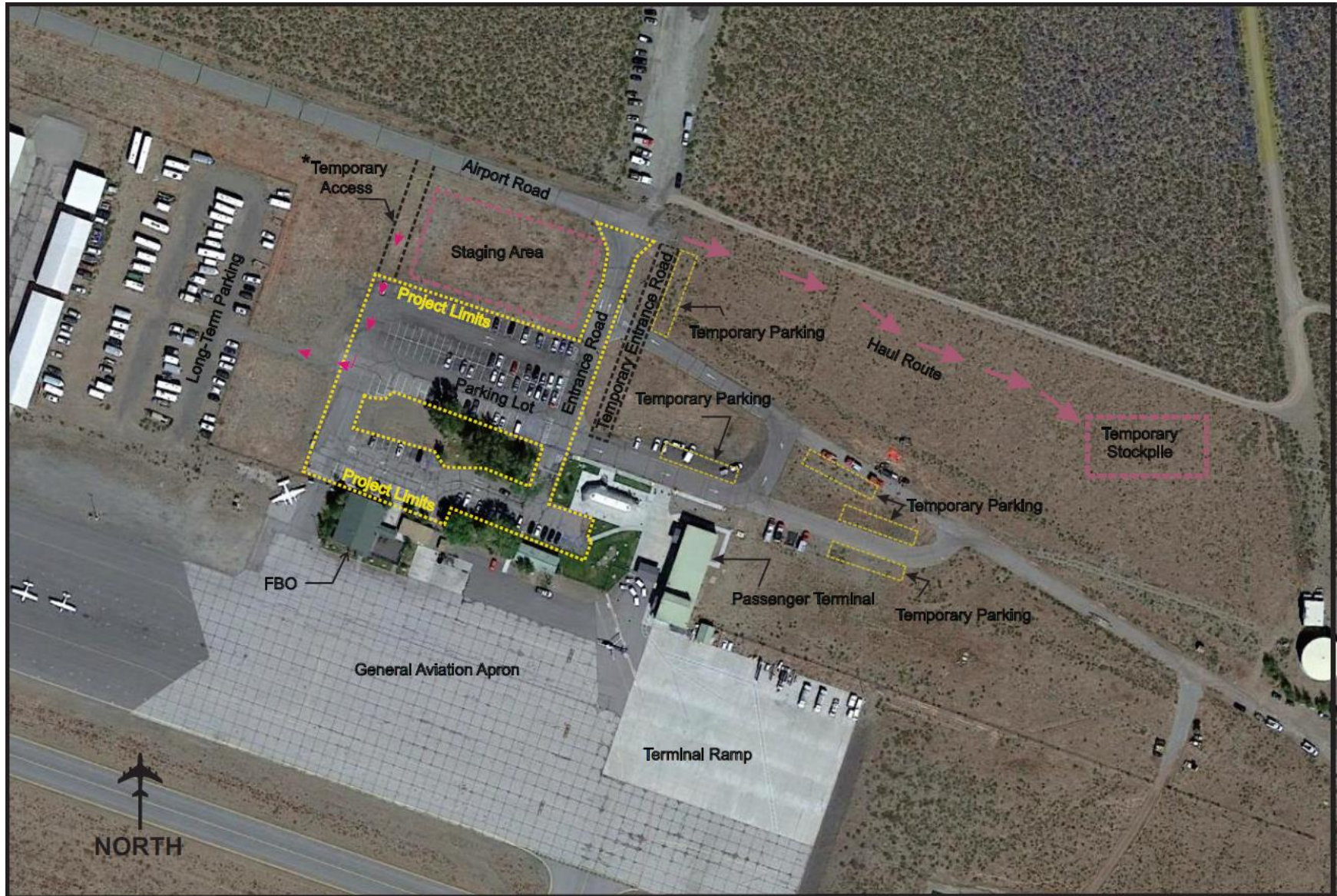
Map of the General Aviation and Terminal Parking Lot Reconstruction Project at Mammoth Yosemite Airport
